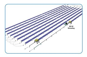
Two AIVs and an ARV are shown above completing ten tracker-rows within a nominal 500MW project – @ rate of over 5,300 panels per 7-hr shift. A second ARV (not shown) would be arriving from the SIF with 2 more re-loads to continue beyond here.
